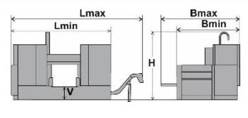
\*L max = chip extractor included, for extractor removal or servis +2700 mm has to be counted with
